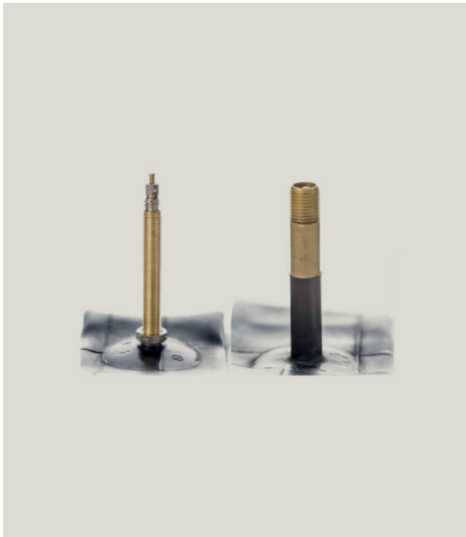
FIGURE 4. Presta (left side) and Schrader (right side) valves.
